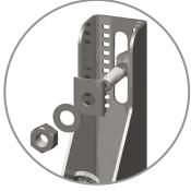
to be halved when rotated through 180° meaning the support level can be finely adjusted by +/- 26.5mm. The design of the Alpha System provides clear inspection into the location and engagement of the washer in the bracket simplifying the final site installation checks.
